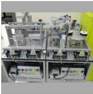
A close-up of two additional Sun Corp. trainers used to teach industrial automation.
