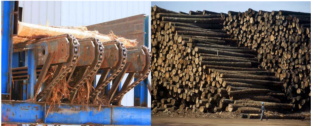
(left) Chain Conveyor (right) Log Deck.
